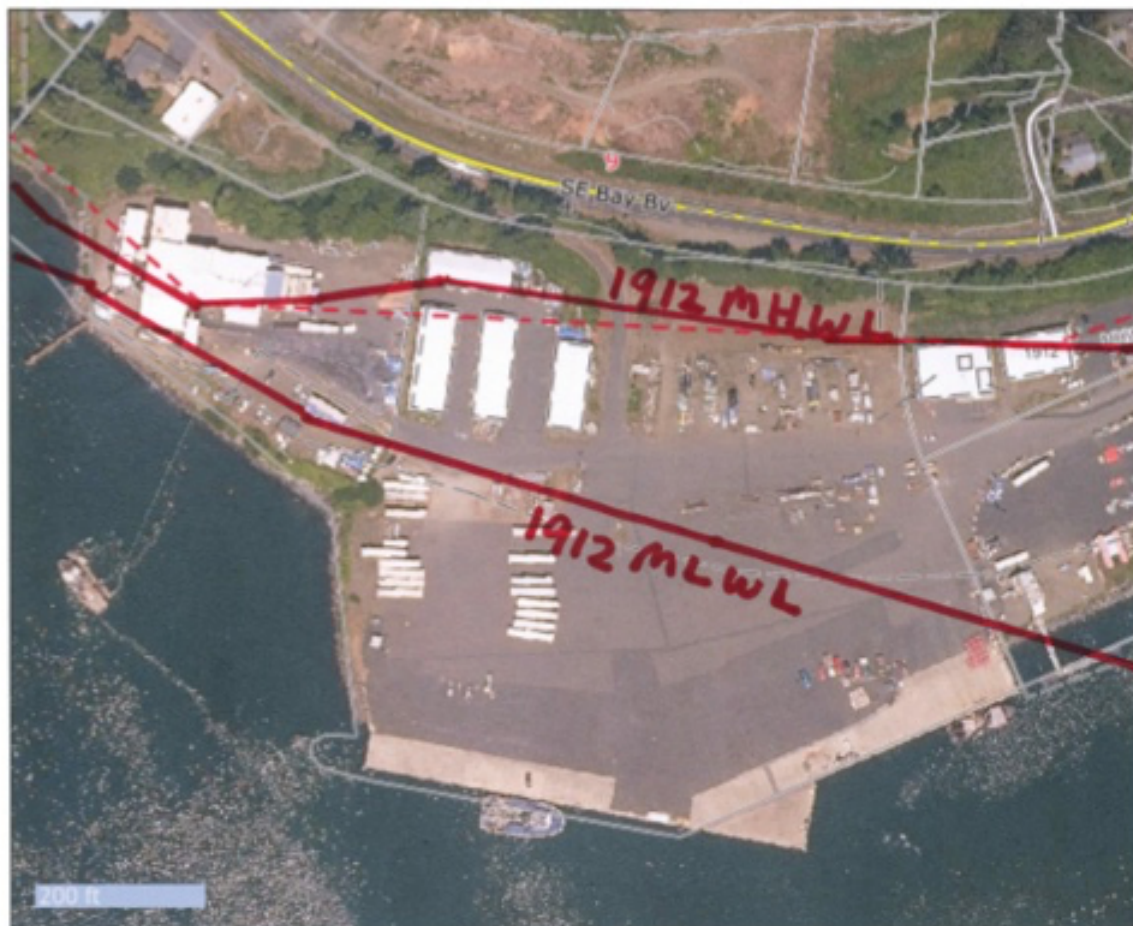
1912 MHWL and MLWL drawn approximately as shown on Lincoln County survey map for Section 9 (Township 11 South, Range 11 West, Willamette Meridian).
