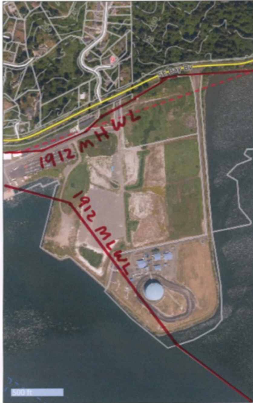
1912 MHWL and MLWL drawn approximately as shown on Lincoln County survey map for Section 9 (Township 11 South, Range 11 West, Willamette Meridian).
